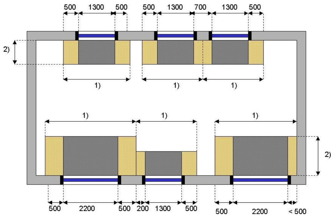
Figure 6 : Part of the floor area behind transparent and non-transparent facade parts that belongs to the daylight area
