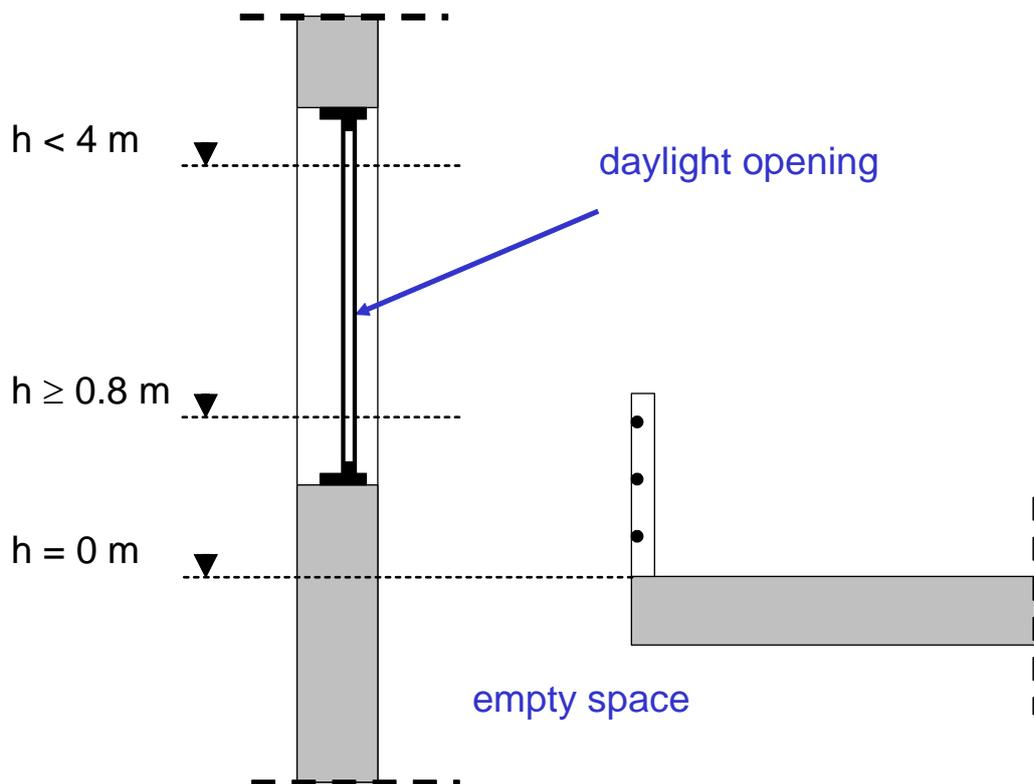
Figure 4 : Projection from the upper edge of the floor to the facade (e.g. with empty spaces) and limitation of the minimum and maximum height to be considered of the (equivalent) vertical daylight opening
